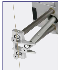
Outer rollers tilt back for easy material acquisition
