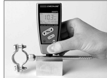
Measurement on cylindrical areas
