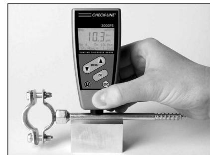
Measurement on cylindrical areas
