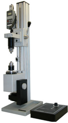
TSTM Motorized, Torque 100 lbin
