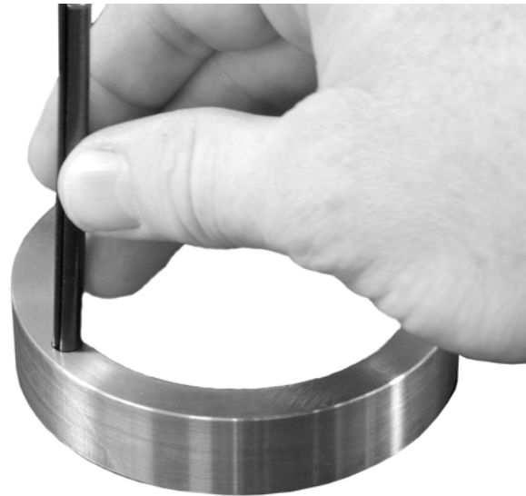
Figure 12 Inserting roll pin
